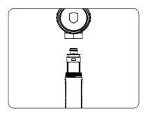
Insert the filter cartridge in the positive direction, keep the visual window to show the filtering effect clearly.
