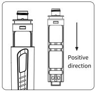
According to the first using date, select the appropriate month number(6 months later) and stick on the replacement indicator window (The cartridge lifetime will be shortened if the quality of local water is poor).
