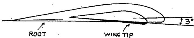
FOR TAPERED WING, ALLOW 3° DOWNWASH AT WING TIP. THIS WILL CAUSE ROOT TO STALL FIRST, THUS RETAINING AILERON CONTROL
