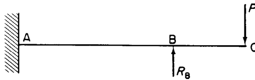
Fig. 5.11 Analysis of a propped cantilever by the method of complementary energy.
