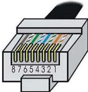
Fig 5.1 Pin Configuration of Type T-568B RJ45 Plug
