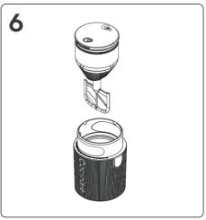
6. Having the ingredients ready in the bowl, place the mixer (with the motor head) into the bowl by aligning the slots of the operating window.
