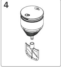
4. Attach the mixing rod to the motor part.
