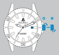
Unscrew the crown counterclockwise until it spins freely (position 0), then pull the crown out to the first click (position 1).
