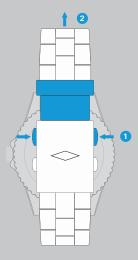
Your watch is equipped with a ratchet style wetsuit extension. This will allow you to determine the amount of extension needed with the push of a button.
