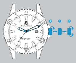
Unscrew the crown counter-clockwise until it spins freely (position 0), then pull the crown out to the second click (position 2).
