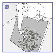
10 Make sure the solid floor is dry, clean and free of any surface contamination. Comb out a continuous layer of cementbased flexible tile adhesive to the underside of the Sloping Board using a 5mm notched spreader.
