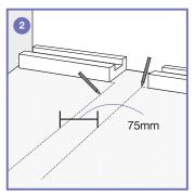
Position the Polystyrene installation supports against the wall and draw around them. Also, indicate the drain position.
