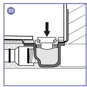
23. Remove the grate and install the riser blocks to bring the grate level with the tiles. Position the grate within the frame.
