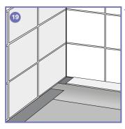
19. Tile the walls down to the Sloping Board and to the drain. Grout the tiles when the adhesive is cured
