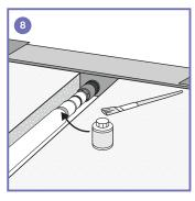
8. Bond the drainage pipe connector to the waste pipe using a suitable solvent weld.
