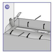
12. Fully unfold the waterproof membrane and draw around it against the walls and Sloping Board. Cut out the corners of the membrane.
