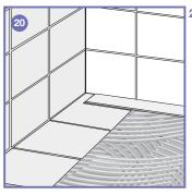
20. Comb out a layer of cement-based flexible tile adhesive onto the Sloping Board and fix the floor tiles up to, around and against the Polystyrene Tile Guide. Grout when the adhesive has cured.
