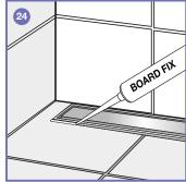
24. Apply a bead of mould resistant silicone sealant to the gap between the grate frame and tiles.
