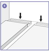
6. Press the Polystyrene installation supports into this recess. Use a spirit level to check the supports are level – and remember that the drain body when installed must be flush with the surrounding solid floor. Allow the adhesive to cure.
