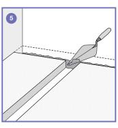
Lay a bed of cement-based flexible tile adhesive in the recess cut for the drain body.
