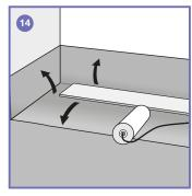
**14.** Press the waterproof membrane onto this adhesive bed, insert the tile guide, and roll it on for a firm adhesion.
