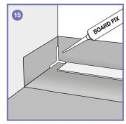
15. Apply Jackoboard Board Fix Adhesive and Sealing Agent to the corners of the Waterproof Membrane.
