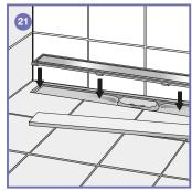
21. Once the grout has cured remove the Tile Guide and drop the frame and grate into position.
