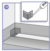
**16.** Apply Board Fix Adhesive to the backs of the PVC Corner Seals and bond them into position.
