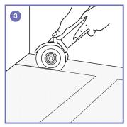
3. Remove the installation supports and following the lines drawn cut a channel for the drain to a depth of 60mm.
