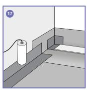
17. Now seal the joint between the Sloping Board and the previously applied Jackoboard Plano Wall Boards with an appropriate sealing system. This could be the Jackoboard Waterproofing and Sealing Set for example.
