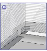
18. Protect the Sloping Board with a sheet of plywood (for example) and comb out a layer of cementbased flexible tile adhesive onto the wall boards with a 5mm notched spreader
