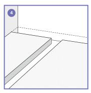
4. Now cut a channel from the drain position indicated deep enough to take a 1.1/2" BSP waste pipe to a suitable exit point. Make sure you allow for a suitable fall in this pipe (3%).
