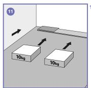
11. Carefully position the Sloping Board up to and around the drain flange and below the waterproof membrane and press firmly down. Place 10-20kg of weight evenly over the Board and allow the adhesive to cure.
