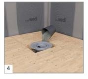
Reinsert the sections of flooring. Fill the box work element with mortar up to the upper edge of the drain flange. Ensure that the mortar is laid as a solid bed in the area around the drain.
