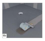
If there is no wedi 610, seal all joints, transitions and holes with the Fundo sealing set.
