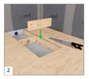
Incorporate the box work element in the area where the drain body will later be fitted. Allow a recess for the pipe.
