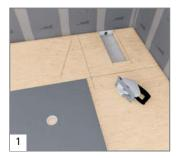
Cut out the required piece of flooring in order to incorporate the drain element.
