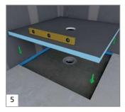
Check drain position by loosely placing the wedi Fundo element and, if applicable, adjust drain position by adding new levelling screed.
