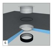
Fit the O-ring from above into the plastic frame and screw down the shower base screw valve into the seal insert.
