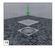
Insert the stainless steel grid. The syphon can be removed and cleaned any time.
