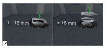
Adjust the grid frame to the height of the top of the tiles including tile adhesive. With a tile thickness of more than 15 mm, the extensions piece will need to be used for height adjustment.
