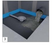
Fill the recess with a bonded levelling screed or slightly moist screed.
