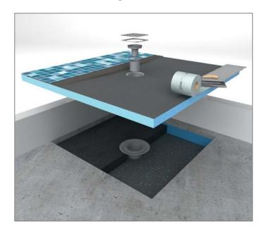
Fundo floor elements from wedi offer a reliable and efficient solution for the construction of waterproof, floor level showers. Featuring a fitted and sealed floor drain, a supplementary factory applied waterproof coating and a predefined slope, they require far less work on any building site and therefore save the construction company a lot of time. Installation with a horizontal drain is demonstrated below.
