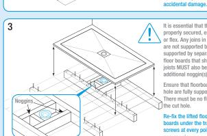
It is essential that the floor boards are properly secured, ensuring no movement or flex. Any joins in the floor boards that are not supported by a joist must be supported by separate noggin(s). Any floor boards that show flexing between ioists MUST also be supported by additional noggin(s).
