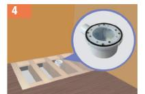
Connect the trap body to your outlet pipework, position between joists and centrally beneath the hole in the ShowerDec®.
