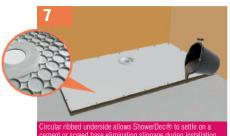
Carefully place ShowerDec® into position. Checking levels in both directions, gently tap ShowerDec® down until level on all 4 sides. It may be necessary to add more self levelling screed, do this by slighlty lifting ShowerDec® & pouring in the screed. Gently tap again until level on all 4 sides.
