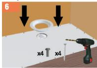
Attach flange to the trap body using the 4 bolts provided, ensuring that the rubber seal is in place. Secure flange to ShowerDec®, there are 4 countersunk indentations in the flange to assist with this.
