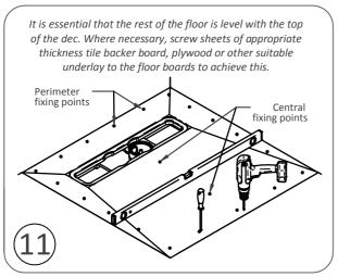
Ensure the dec is perfectly level, then drill and screw it to the plywood beneath using screws provided (5x60mm). The dec should be secured around the perimeter at approx. 200mm intervals and in the centre as shown.
