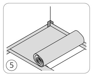
Measure and cut required length of Waterguard Membrane. Remove the release paper and carefully set into position - pressing firmly onto the jointing tape. Repeat steps 4 and 5 untill the floor is covered.
