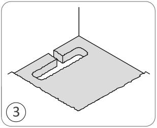
Mark a position of the drain channel and remove enough concrete for the installation of a waste pipe and shower trap. It is important that there is suitable support for the base of the trap, 96mm below the level of the bottom of the dec.
