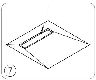
Place the dec onto the plywood platform. Mark a line around the aperture in the dec into which the drain fits.
