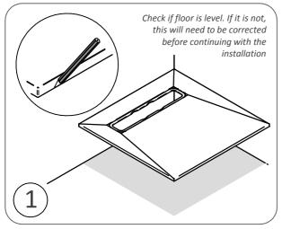
Position the Aqua-Dec Linear in the desired location on the floor and mark around the outer edge.
