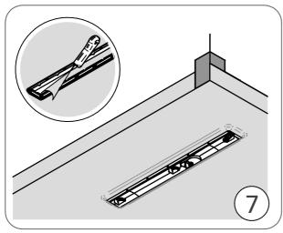
Find the location of the drain by gently pressing the membrane over the drain channel, then using the membrane clamp as a guide, cut the membrane to the inside edge and remove centre piece.
