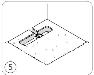
Lay a weak sand cement mix in the excavated hole. Ensure the mix is fairly dry.
