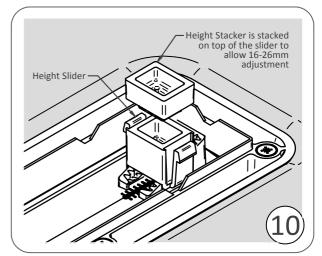
The correct height of the tile frame assembly is achieved by moving the height slider into the corresponding position in the ramp (6-16mm). To gain an additional 10mm, the height stacker is stacked on top of the slider.
