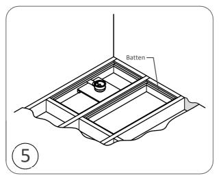
Fix battens to the side of the joists and noggins. The battens must be fixed 18mm below the top of the joists to allow for the thickness of the plywood to provide flat and level base on which the dec will be installed.
