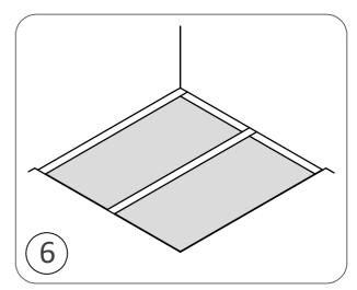
Measure and cut out 18mm plywood panels. Position them, but DO NOT SECURE YET. Check the panels are level with each other.
