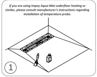
Ensure the surface is clean, dry, free from dust, grease, oil etc., all indentations should be filled and any protrusions struck off. Oily or greasy surfaces should be cleaned with a suitable cleaner, thoroughly rinsed then allowed to dry. Apply the primer to all porous surfaces.
