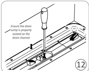
Position the drain channel into the dec and screw it to the drain sump as shown. **Do Not Overtighten.** Then using an appropriate drill, drill through and screw it to the dec in the predefined positions on the top of the drain channel.
