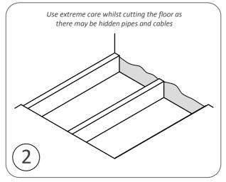
Using suitable saw, cut along the outline, then remove the floorboards.
