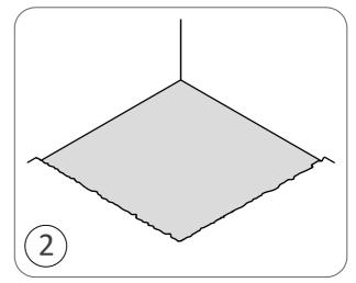
Using a suitable equipment, excavate all the concrete within the marked area to a minimum depth of 35mm. Use extreme care whilst cutting the floor as there may be hidden pipes and cables.
