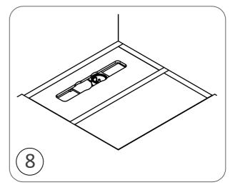
Using a suitable saw cut along the outline previously drawn onto the plywood base. If the lines cross the joists, notch the joists in accordance with current building regulations to a maximum depth of 20mm (this may be reduced if the dec needs to be packed up).
