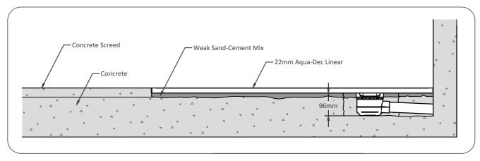
Diagram 3. Cross section of Dec and concrete floor.
