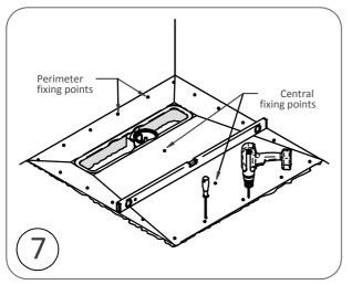
Ensure the dec is perfectly level, then drill and screw it to the concrete below using suitable sized plugs and screws. The dec should be secured around the perimeter at approx. 200mm intervals and in the centre as shown. **Ensure the dec does not become distorted when screwing down.** Leave to set over night.
