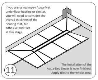
When the linear drain cap is inserted it should be level and flush with the tiles. Once the desired height is determined the height sliders/stackers must be glued in place with an ABS suitable solvent cement.
