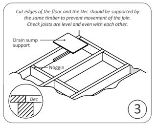
Fit noggins and trimmers to support outer edges of the Dec. A support 96mm below the level of the bottom of the dec should also be fitted at this point. This is for the drain sump to rest on.
