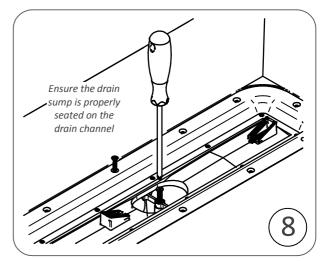
Position the drain channel into the dec and screw it to the drain sump as shown. **Do Not Overtighten.** Then using an appropriate drill, drill through and screw it to the dec in the predefined positions on the top of the drain channel.
