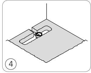
Measure where the drain sump would appear once in position. Place it in the excavated area ensuring the base is sufficently supported, then install the waste pipework in accordance with current building regulations and connect to the trap using solvent cement.
