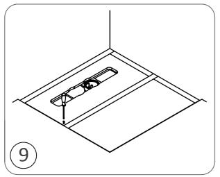
Drill and screw the plywood base to the battens below.
