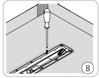
The clamp should be carefully pressed into position to allow the membrane to stretch over the linear channel, once the membrane has begun to stretch into place, gradually tighten the screws. The clamp must be lowered evenly into place. **Do not use power tools.**
