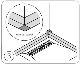
Using the 150mm jointing tape, line all the corners and wall/floor junctions so that the tape overlaps 75mm at the wall and 75mm onto the floor.
