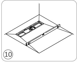
Replace the dec onto the plywood base, ensuring it is perfectly level. This is important if the correct drainage from the dec is to be achieved. If this is not the case, use suitable packing under the dec to ensure it is level.
