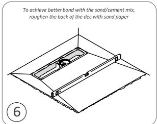
Place the dec onto the weak sand/cement mix ensuring the dec is flush with the surrounding floor and perfectly level. If this is not the case pack more weak sand/cement mix under the dec.
