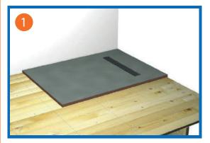
1) Clear the working area, establish where you want to fit the WetBase tray and place the tray on top of the floor boards. Mark around the tray with a pencil and draw the position of the waste hole.
