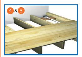
4) Build a support for the trap with a plywood platform approx. 110mm down from the top of the joists, for the drain assembly to sit on, to prevent the drain from dropping after fitting. Test fit the trap assembly and ensure correct alignment before
