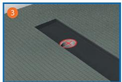
3) Identify the best position for the drain trap assembly. The linear drain offers a choice of three trap positions, left, middle or right, so joists can be avoided.
