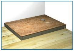
If you cannot set the tray level into the floor and have to raise the base up, for example to accommodate above floor drainage we suggest you construct a 75mm x 50mm support frame on top of the floor to the overall size of the wetroom area and cover in 18mm ply. Then lay the WetBase® on top and secure with flexible tile adhesive.
