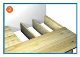
2) Remove the floor boards from the area where the tray is to be fitted. Ensure you take the floor boards back to the centre line of the nearest joist to ensure maximum support. You may have to refit some of the floor boards around the tray to ensure a snug fit.
