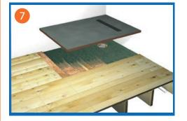
7) Test fit the WetBase® Linear Universal tray to ensure a tight fit and alignment with the drain. Apply a thin bed of flexible tile adhesive to the platform you have constructed using a notched trowel. Fit the tray over the bed of adhesive and firm down ensuring the tray is level in all planes. Carefully weigh the corners of the tray down (using bags of adhesive / tiles etc) to help ensure a full and level adhesion.
