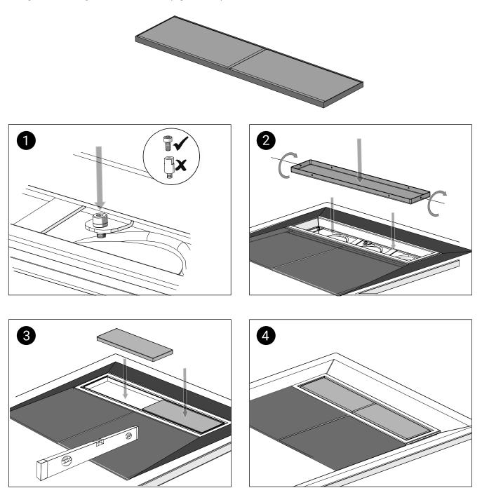
Note: Tiles should only be used to cover the former. Measure all angles and distances for tiles around the gully and ensure there is a slope of between 2% and 4% to the trough outlet.
