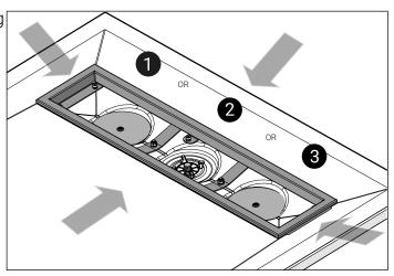
If not all waste holes are needed, plugs are supplied to fill in the recess to prevent water collecting. Plug guides – the plugs have drill guides in the centre to help installers drill the waste hole centrally.
