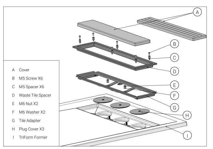
**TriForm has 4 fall planes** effectively directing the water into the waste giving a high flow rate and complete level access.
