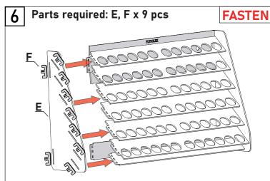
Install the second E part as shown on the scheme. You can flip the organizer vertically for more convenience. Fasten the installed part using elements F (as in step 2).
