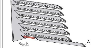
Fasten inserted parts using elements F.
