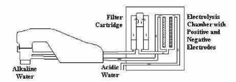
A special attachment re-directs tap water out of the faucet through a plastic hose into the lonized Water unit. Inside the lonized Water unit, the water is first filtered through activated charcoal. Next, the filtered water passes into an electrolysis chamber equipped with a platinum-coated titanium electrode where electrolysis takes place.
