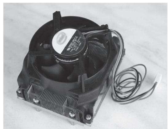
A CPU produces much heat. A fan (shown) prevents overheating.
