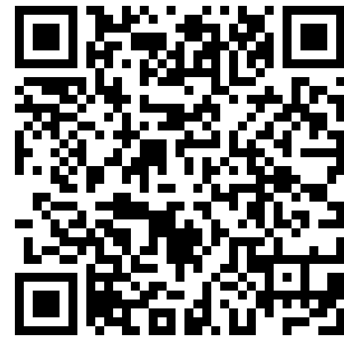
Mobile tag. Take a picture of this tag using your mobile phone. Are you able to read the text? It should read: 'Hello ITGS student! This text is encoded in the mobile tag.' The three squares help the software to orient the mobile tag for decoding.
