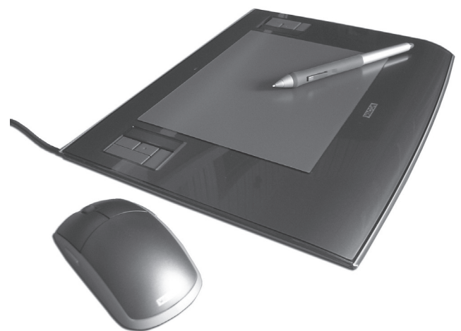
Graphics tablets can be used as an alternative to mouse input and are commonly used by people who do graphics-intensive work.
