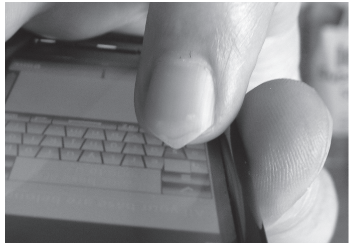
Touch screens combine an LCD display with a pressure-sensitive surface. The user can interact directly with the computer by touching the different regions on the screen.
