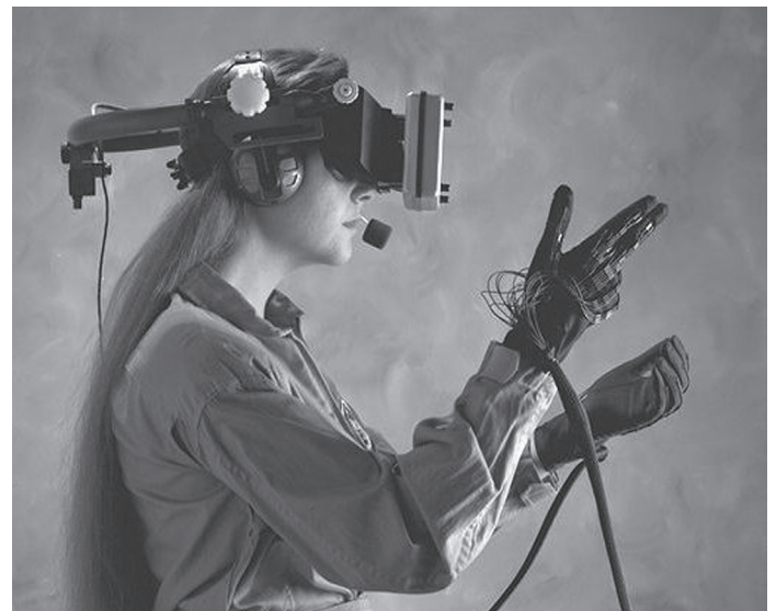
Virtual reality (VR) interfaces submerge the user in a computer-generated environment. This picture shows VR gloves (input interface), VR goggles (output interface) and a microphone (input interface).
