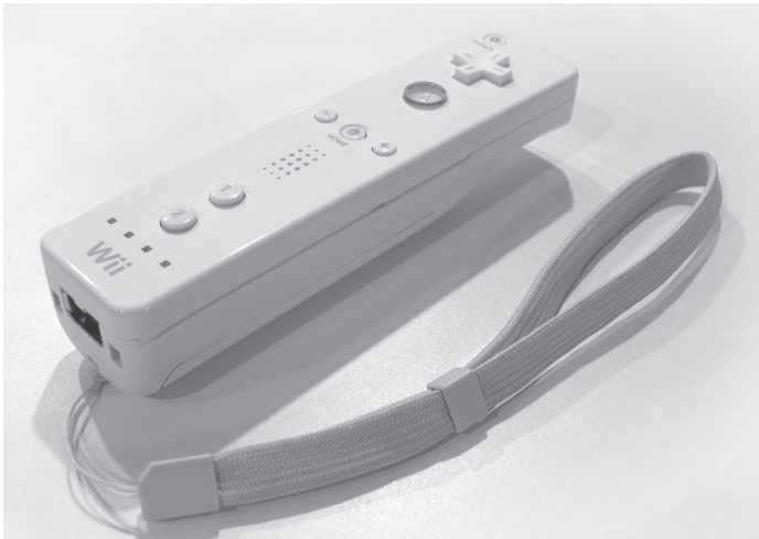
Wii game controller. This game controller combines a motion sensor with push buttons.
