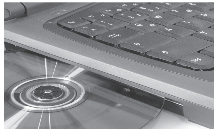
Optical drive. CD-ROMs and DVDs are read by a laser beam.
