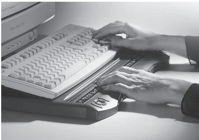
Braille output. This output device is a computer-human interface that enables blind people to read.
