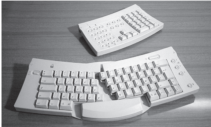
An ergonomic (split) keyboard allows the user to type without bending the wrists outwards.
