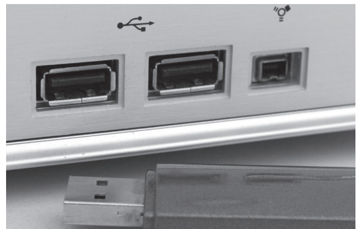
The fast USB port of the PC is compatible with the slow USB flash memory stick. The port will adjust its transfer speed so that the stick is able to handle the input.
