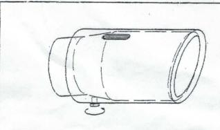
4. While maintaining chromed exhaust tip in this position, tighten bolt until contact occurs with tailpipe.
