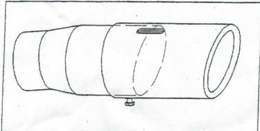
Position chromed exhaust tip over tailpipe with bolt facing down.
