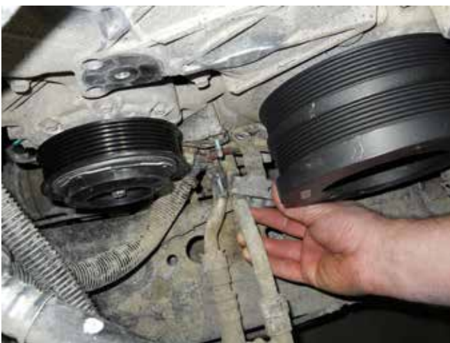
5. Use a cut-off wheel to cut the stuff off at the base.
