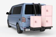
The box holder is used to attach a transport box or other equipment (e.g. large travelling bag or sports equipment).
