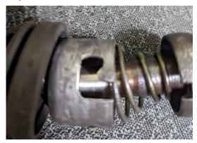
Put the transmission into neutral. Remove the stock shifter by pushing down on the cup, and with a flat screwdriver, hitting the screwdriver (with your palm or a hammer) counter clockwise to release the lock pins.
