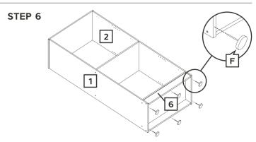
Attach leg studs (F) to bottom side of side panel left (1), side panel right (2) and 2 x support panels (6) using a soft headed mallet.
