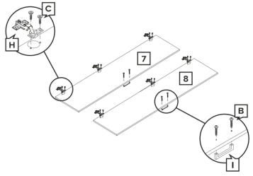
Attach metal door hinges (H) to door panel 1 (7) and door panel 2 (8) using fine thread medium screws (C). Attach handles (I) to door panel 1 (7) and door panel 2 (8) using medium pan head screws (B). Make sure handle is on opposite to the hinges.
