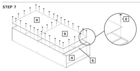
Attach back panel (9) to side panel left (1), side panel right (2), top panel (3) and 2 x fixed shelf panels (4) using nails (E), and gently tap in using a soft headed mallet.
