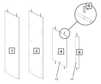
Insert wood dowels (G) into pre-drilled holes in side panel left (1), side panel right (2),  $2 \times 1$  fixed Shelf panels (4) and  $2 \times 1$  support panels (6) as shown above.
