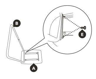
Attach left leg to underside of seat by using 14mm screw (E) but do not tighten.
