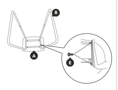
Attach right leg to underside of seat by using 14mm screw (E) but do not tighten.
