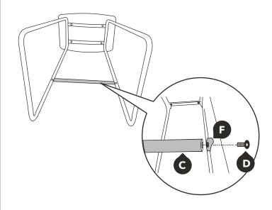
Attach the foot rail to the legs by using 35mm screw (D) but do not tighten.
