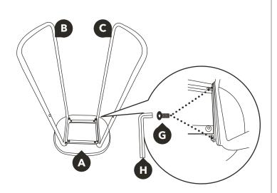
Attach right leg to underside of seat by using (Gx2) screws but do not tighten.
