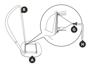
Attach left leg to underside of seat by using (Gx2) screws
