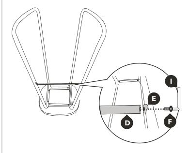
Attach the foot rail to the legs by using (F) screws and (E) nuts but not tighten.
