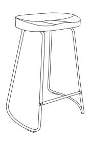
Place the stool on level ground and then check if it is stable. If not, please adjust metal legs until it is stable. Once stable, tighten all screws.
