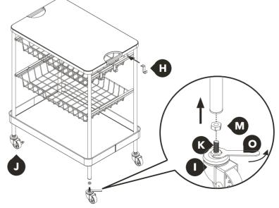
Screw the nuts (M) onto the threaded shaft of each wheel, then screw the wheels into the bottom of the left and right ends. Use the spanner provided to tighten. Ensure the two braking wheels are both attached to the same end. Hang the utensil hooks onto the frame to complete the assembly.
