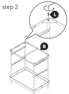
Use the hex key provided to secure the top frame to the left and right ends using the hex bolts.
