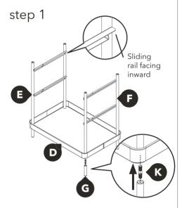
Use the double ended bolts to secure the legs to the left and right ends through the base tray. Ensure that the sliding rails are facing inwards.
