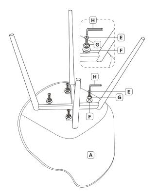
Attach Seat (A) to frame assembly using 4x short hex screws (E), 4x spring washers (G) and 4x washers (F). Tighten using the allen key (H).
