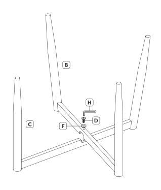
Attach frame (C) to frame (B) using 1x long hex screw (D) and 1x washer (F). Tighten using the allen key (H).
