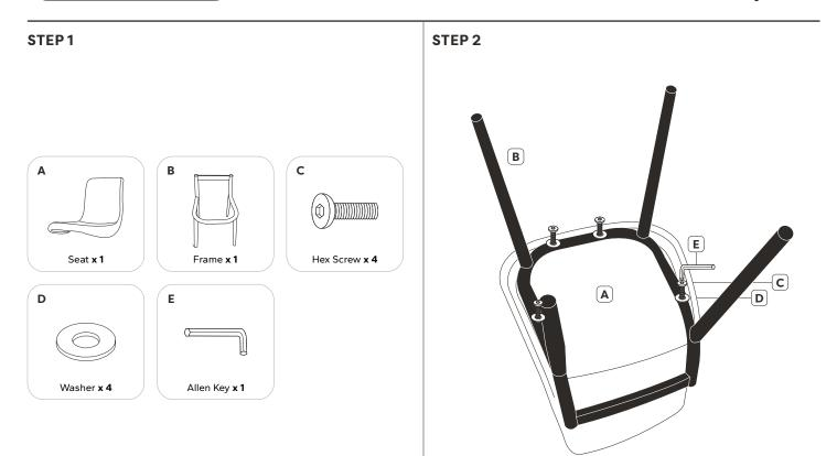
Attach Seat (A) to Frame (B) using 4x Hex Screws (C) and 4x Washers (D). Tighten using the Allen Key (E).
