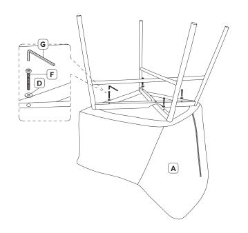
Attach Seat (A) to frame assembly using 4x long hex screws (F) and 4x washers (D). Tighten using the Allen Key (H).
