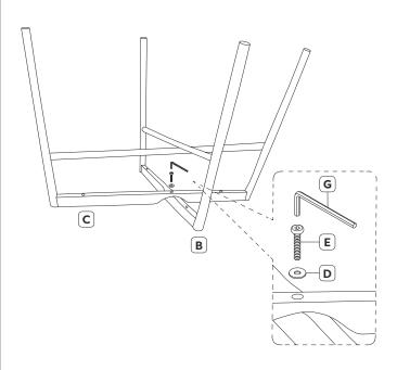
Attach frame (B) to frame (C) using 1x short hex screw (E) and 1x washer (D). Tighten using the allen key (G).
