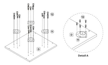
Attach 4x leg mount plates (11) to bottom panel (D) using pan head screws (12).
