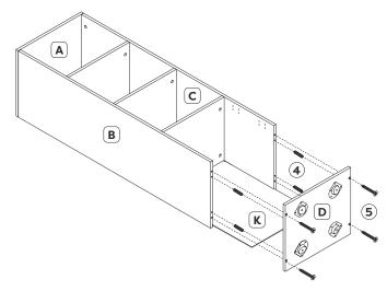
Slide bottom back panel (K) into the grooves in side panels (B and C) and middle shelf panel (E). Insert medium wood dowels (4) into pre-drilled holes in side panels (B and C), align bottom panel (D), and slide into position. Fix bottom panel (D) using long flat screws (5).
