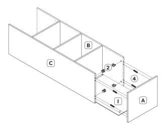
Slide top back panel (I) into the grooves in side panels (B and C) and middle shelf panel (E). Insert medium wood dowels (4) into pre-drilled holes in side panels (B and C), align top panel, and slide into position. Insert cam nuts (2) into pre-drilled holes in side panels (B and C), ensuring arrows point towards top panel (S). Tighten using a phillips head screwdriver.
