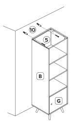
Move the assembled unit to its final position, and fasten into wall using wall plugs (10) and long flat screws (5) provided, or other suitable hardware to securely fix the unit to your wall. Seek advice from a qualified trades person on how to secure the unit to your specific wall. We strongly advise that you secure the unit to a wall to prevent the unit from toppling.
