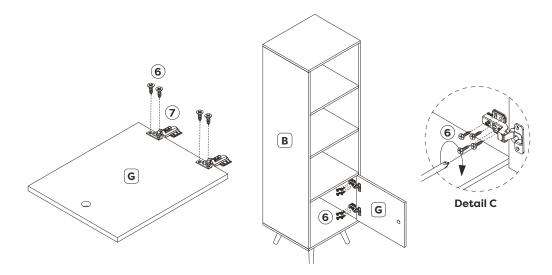
Attach door hinges (7) to door panel (G) using short flat screws (6). Fix door panel and hinges To the assembly using short flat screws (6), per detail C.
