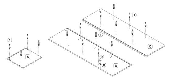
Insert cam bolts (1) into pre-drilled holes of side panels (B and C) and top panel (A) as shown. Attach door stop (8) to side panel left (B) using small flat screws (9).
