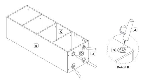
Attach legs (J) to bottom panel (D) by screwing into leg mount brackets (11) previously fixed to the bottom panel (D).
