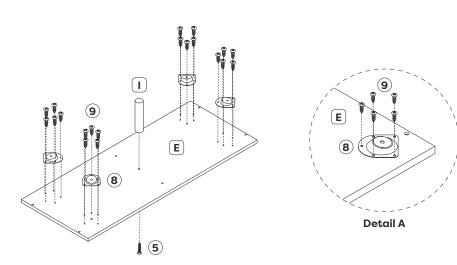
Fix 4x leg mount brackets (8) to bottom panel (E) using small dome screws (9) per detail A. Attach central leg (I) to bottom panel (E) using a long flat screw (5).
