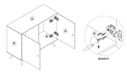
Attach door panels (G) to the assembly using 4x short flat screws (6) per hinge.
