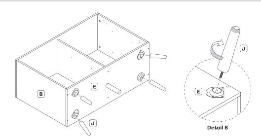
Attach angled legs (J) to bottom panel (E) by screwing into leg mount brackets (4) previously attached to the bottom panel.
