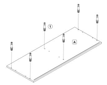
Screw cam bolts (1) into pre-drilled holes in top panel (A) as shown.
