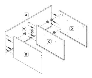
Insert wood dowels (3) into the pre-drilled holes in centre panel (C) and side panels (B and D). Align cam bolts and wood dowels with pre-drilled holes and place top panel (A) in position. Insert cam nuts (2) as shown, with arrows pointing towards the top panel, then tighten cam nuts (2) using a phillips head screwdriver.
