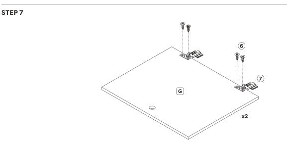
Attach 2x hinges (6) to each door panel (G) using short flat screws (7).
