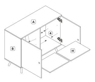
Insert adjustable shelf mounts (4) to the desired pre-drilled holes in centre panel (C) and side panels (B and D), then slide adjustable shelf panels (H) into position.
