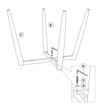
Attach frame (B) to frame (C) using 1x short hex screw (E) and 1x washer (D). Tighten using the allen key (G).
