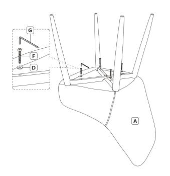
Attach Seat (A) to frame assembly using 4x long hex screws (F) and 4x washers (D). Tighten using the Allen Key (H).
