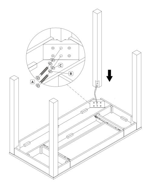
Attach table legs to pre-assembled table top. Using allen key (D) provided, thread washer spring (B) and washer (C) through M6 x 50 screw (A) on centre two holes of leg. Tighten using the allen key (E) provided.
