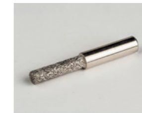
Coarse router 12.7mm diameter shaft / 10mm diameter cutting head. 20/30 grit.
