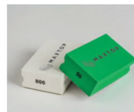
ELECTROPLATED DIAMOND HAND PADS 50 grit coarse pad and 800 grit finishing pad. For sanding quartz edge after sawing or routing process and creating a bevel. (Located under flap inside installation kit box).
