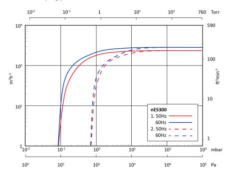
Figure 6 nES300S Pumping performance curve
