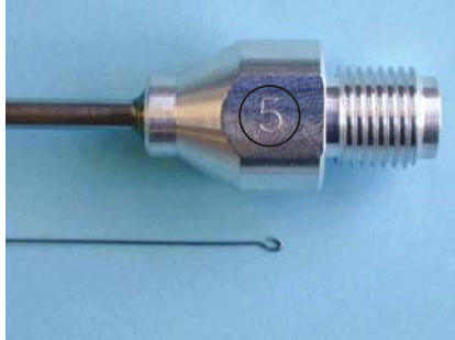
Sniffer probe equipped with a dia. 0.35 mm needle is marked "5".
