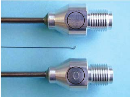
Sniffer probe equipped with a dia. 0.30 mm needle has no mark or is marked "0".
