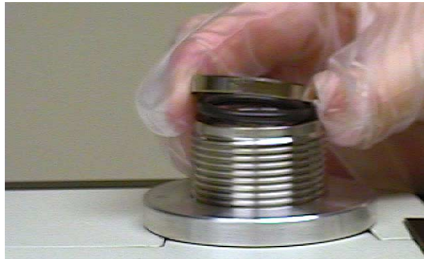
Figure 4-15 Placing the O-ring and Compression Ring onto the Test Port
