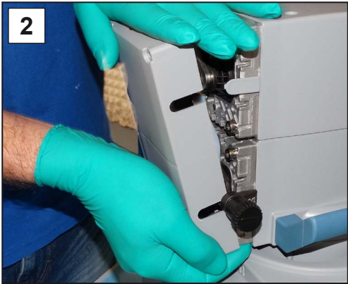
2. Remove the housing cover and lay it aside.
