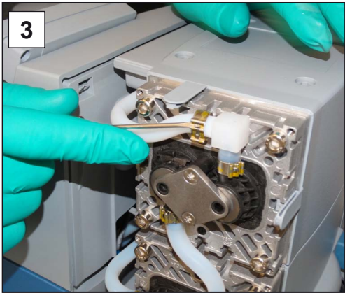
3. Open the hose clamps of the outer hoses. Flat-head screwdriver 1.
