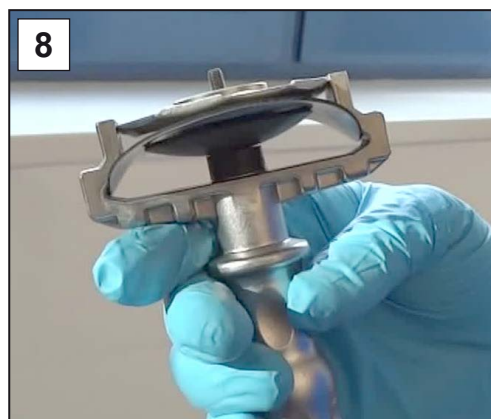
8. Fixate the diaphragm parts inside the diaphragm wrench.
