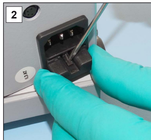
2. Carefully pull out the fuse holder.
