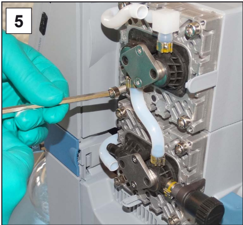
5. Unscrew the socket head screws from the head covers. Allen key 5.
