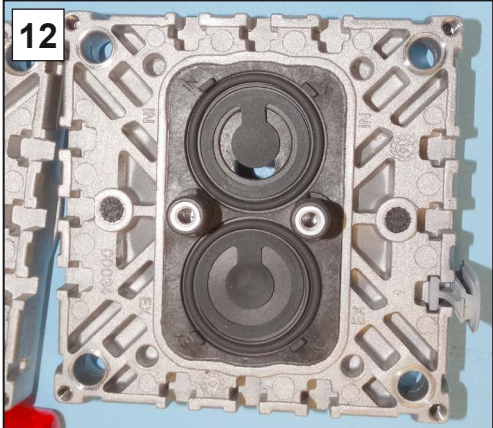
12. Position the new valves and align them.
