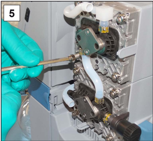
5. Unscrew the socket head screws from the head covers. Hex key size 5.
