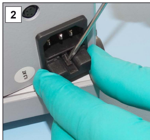
2. Carefully pull out the fuse holder.
