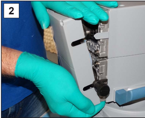
2. Remove the housing section and set it aside.
