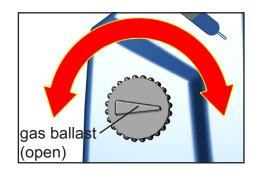
For **condensable vapors** (water vapor, solvents, etc.):
