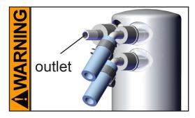
Never block the gas outlet (hose nozzle for tubing I.D. 3/8" (10 mm)). The exhaust hose has always to be unobstructed and without back pressure to enable an unhindered discharge of gases and protect the pump valves from damage.
