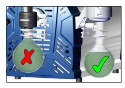
In case of **condensation**: Check the liquid level in the catchpots during operation. Check the liquid level in the catchpots regularly. Do not allow the catchpots to overfill. Drain catchpots in time to avoid overflow. Install a level sensor (see "Accessories / Spare parts", pg. 43) for monitoring, if necessary (VACUUBRAND controller CVC 3000 or VNC 2 is required).
