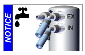
Check all hose connections prior to starting operation of the cooling system.
