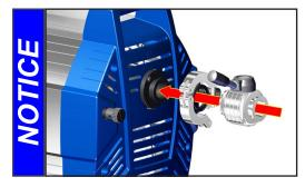
Use a suitable valve (see "Accessories / Spare parts", pg. 43) to isolate the pump from the vacuum application. This is to allow the pump to warm up before pumping condensable vapors and to clean the pump after use before it is switched off.
