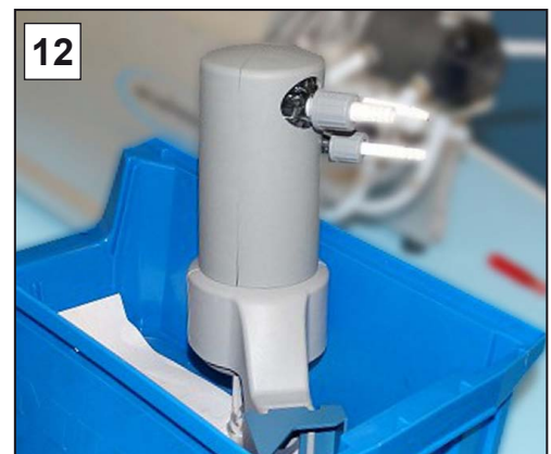
12. Set the chiller down securely so that no liquid can escape.
