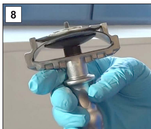
8. Secure the diaphragm assembly inside the diaphragm wrench.
