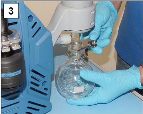
3. Remove the glass flask from the EK as well as the connected hoses.
