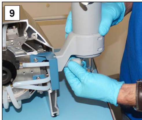
9. Undo the union nut on the EK feed line.
