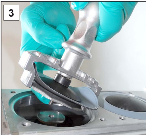
3. Lift the diaphragm, along with all the parts, out of the vacuum pump.
