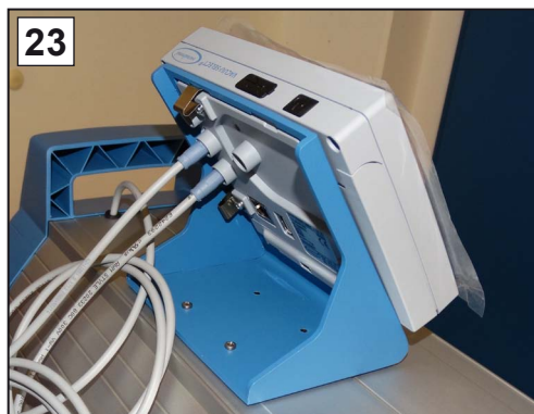
23. Secure the controller on the pumping unit and connect all cables.
