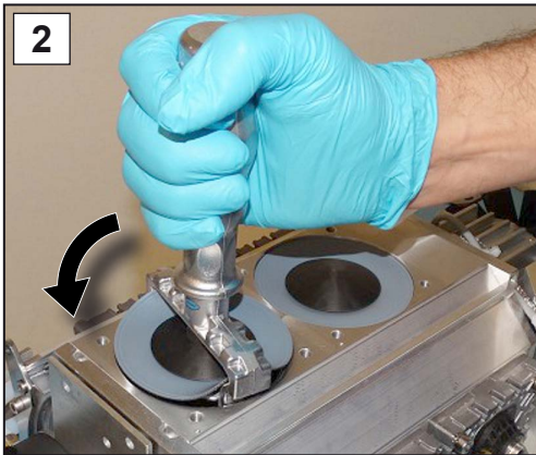
2. Carefully position the diaphragm wrench on the diaphragm support disc and unscrew the assembly with the diaphragm wrench attached.
