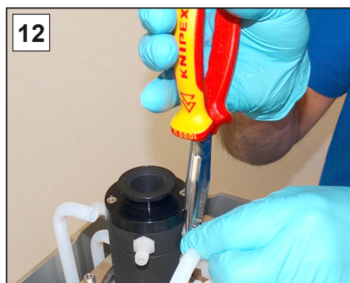
12. Secure the hose clips on the hose nozzles, e. g., with flat nose pliers.
