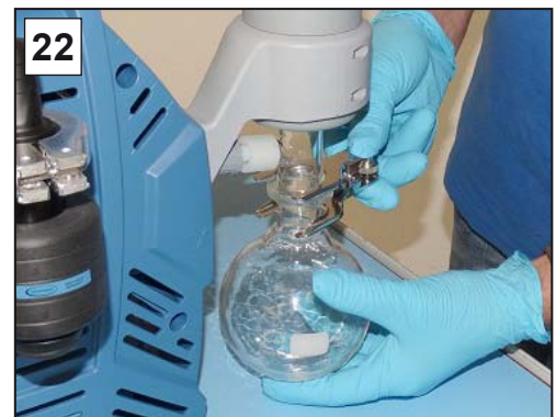
22. Secure the glass flask to the EK.
