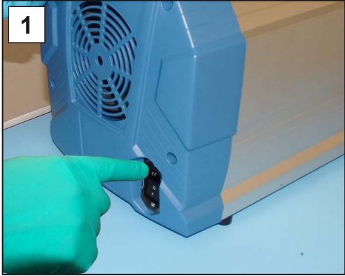
1. Switch the pumping unit off and unplug the power plug.
