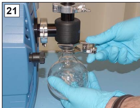
21. Secure the glass flask to the inlet IN.
