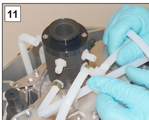
11. Push the molded hoses back into place on the hose nozzles.
