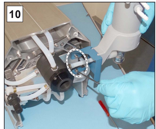
10. Unscrew the 2 screws in the EK holder; hex key size 4.
