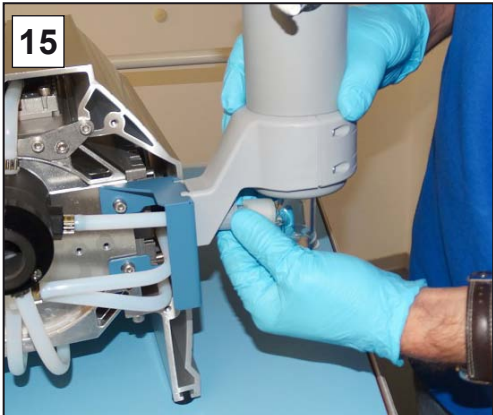
15. Secure the union nut on the EK feed line.
