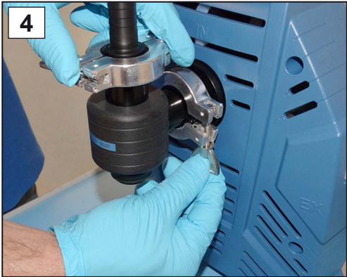
4. Open the clamping ring of the separator flask.
