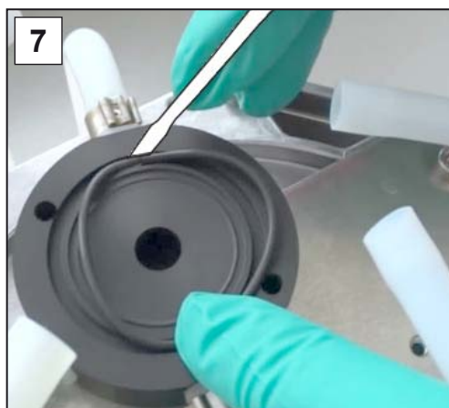
7. Replace the used O-ring.
