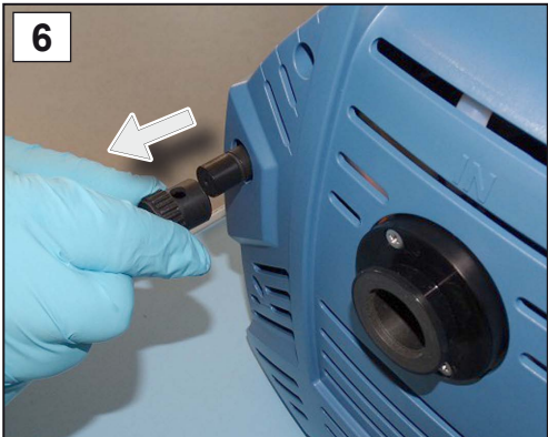
6. Remove the cap from the gas ballast.
