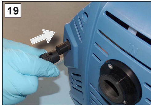
19. Place the cap on the gas ballast.
