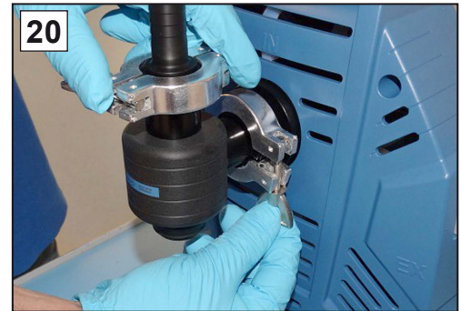
20. Secure the separator flask with the clamping ring.
