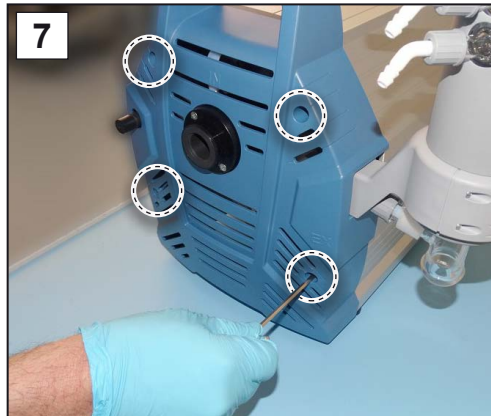
7. Unscrew the 4 screws from the front housing section; hex key size 4.
