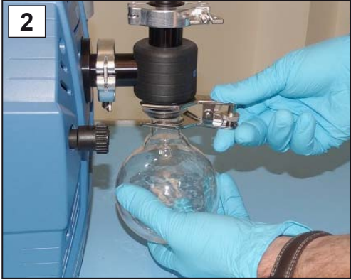
2. Remove the glass flask from the inlet IN.
