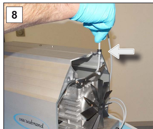
8. Secure the cable in the rear recess.
