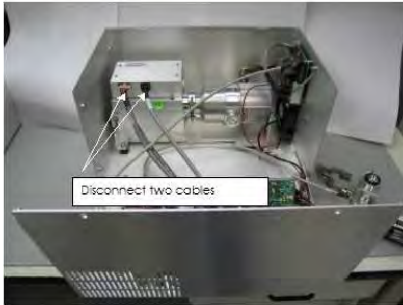
Figure B-49 Cables To Spectrometer
