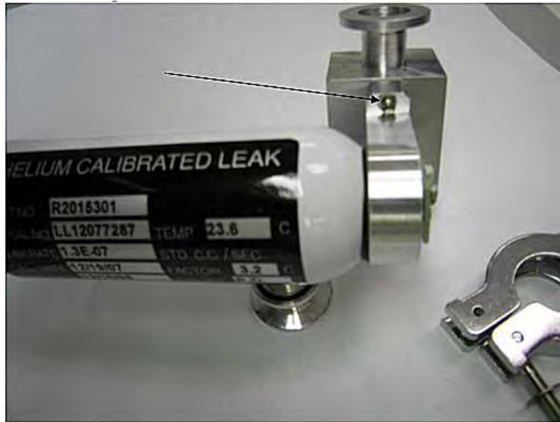
Figure B-44 Calibrated Leak Screws
