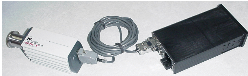
Figure 3: Inficon BPG400 Connected to the Terranova 970
