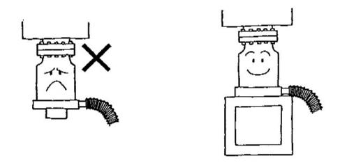
3) Fill the oil sump with oil before starting the HGP.
