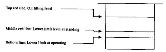
Fill oil to the oil filling level if the level of oil lowers exceeding the given lowest level at standing and operating each.
