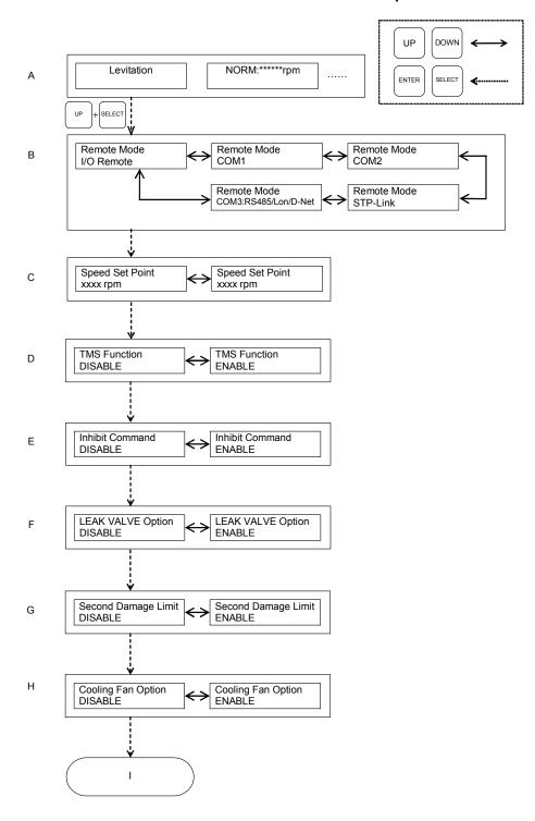
Figure 23 - Parameter setting method
