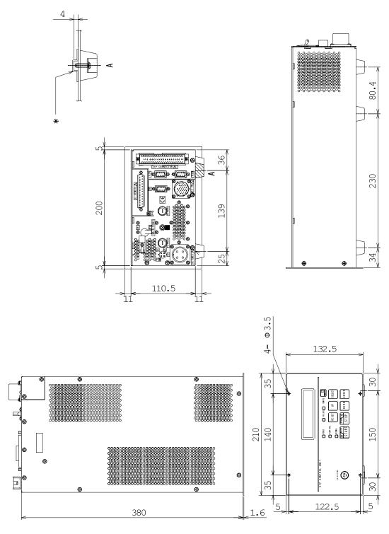
Figure 9 - SCU-800 dimensions (mm)
