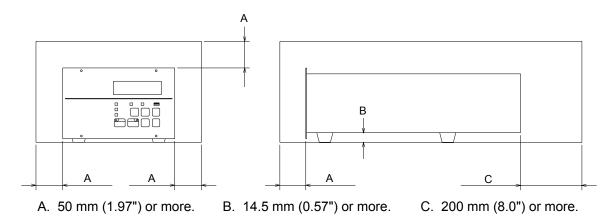
Figure 12 - Installing the SCU-800
