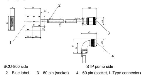
Figure 14 - STP pump connection cable
