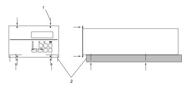
1 Front panel 4 securing screws
