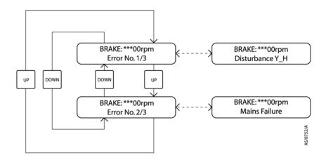
Note: The upper message on the LCD shows the current STP pump operation state. The lower message on the LCD is alternately displayed.
