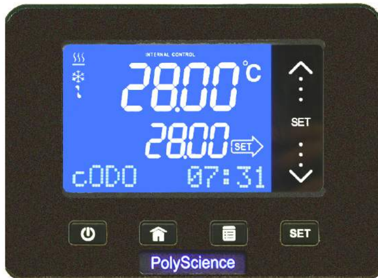
Compressor Operating Time – (shown here in hours and minutes)
