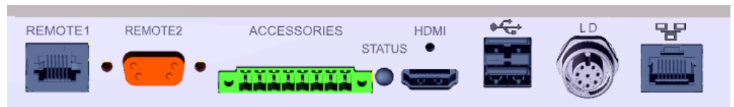
Fig. 5: Connections for accessories and control signals at the back side of the device.
