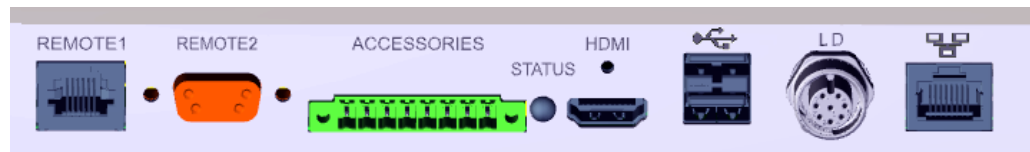
Fig. 4: Connections for accessories and control signals at the back side of the device.
