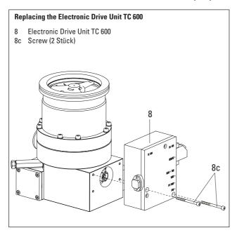
→ Install the new Electronic Drive Unit TC 600 back onto the turbopump and connect again.
