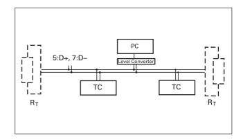
All units connected to the bus must have differing serial interface addresses (parameter 797).
