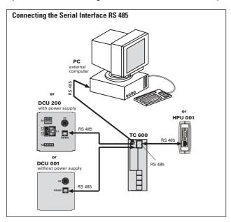
The serial interface is galvanically and safely separated from the maximum supply voltage from the TC 600.
