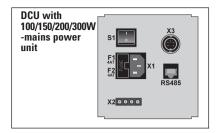
S1 Mains switch F1 Mains fuse F2 Mains fuse X1 Mains connection 90-265 V~ X2 Output for voltage supply, electronic drive unit Х3 Pressure gauge connection Communication with electronic drive RS 485 unit
