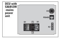
S1 Mains switch F1 Mains fuse F2 Mains fuse X1 Mains connection 90-265 V~ X2 Output for voltage supply, electronic drive unit Х3 Pressure gauge connection RS 485 Communication with electronic drive unit
