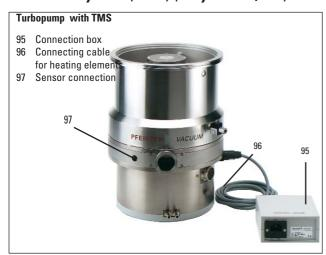
The Temperature Management System (TMS) comprises a regulatable heating system which is installed in the forevacuum part of the turbomolecular pump. Heating up to a maximum of 90°C prevents the condensation of process gases or by-products in this part of the pump.
