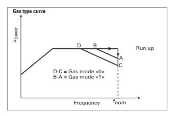
The rotation speed is reduced when the gas dependent maximum power is exceeded until there is equilibrium between the permissible power and the gas friction. To avoid rotation speed fluctuations it is recommended to set (in rotation speed setting mode) the equilibrium frequency or a somewhat lower frequency.
