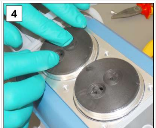
4. Position the new valves and align them; service kit MD 1C.
