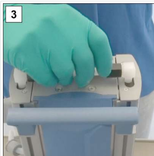
3. Screw on the union nut until it is finger-tight; open-end wrench SW17.
